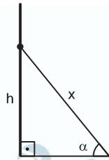
$$\begin{aligned}\text{sen } \alpha &= \frac{h}{x} \\ \Rightarrow x &= \frac{h}{\text{sen } \alpha}\end{aligned}$$
